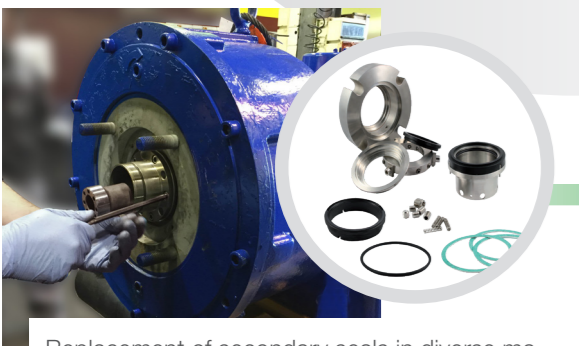
Replacement of secondary seals in diverse materials: NBR, EPDM, EPDMPEOX, FPM, FFKM, AFLAS, HNBR, PTFE, etc.
