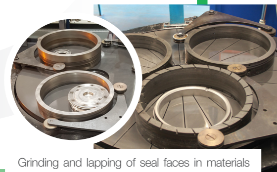
Grinding and lapping of seal faces in materials such as silicon or Tungsten carbide and their manufacture in materials such as graphite, antimony or PTFE.
