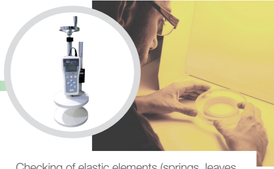
Checking of elastic elements (springs, leaves, Super-sinus springs) and their replacement if necessary, in all cases ensuring the correct force is exerted.
